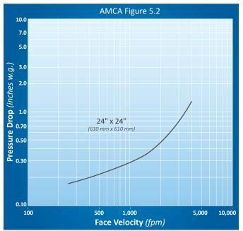
Air Performance testing was conducted in accordance with ANSI/ AMCA Standard 500-D, Figure 5.2. Vertically mounted test damper is located at the end of 5 diameters of a duct run, exhausting into an open area. Both duct and test damper are downstream from air supply.
