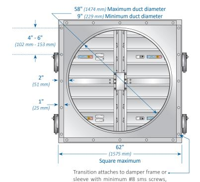
1/4" bolts, 3/16" rivets, or welds.
