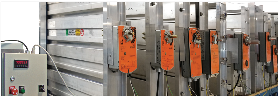
The actuators installed on each damper were connected to a timed electronic cycler.
