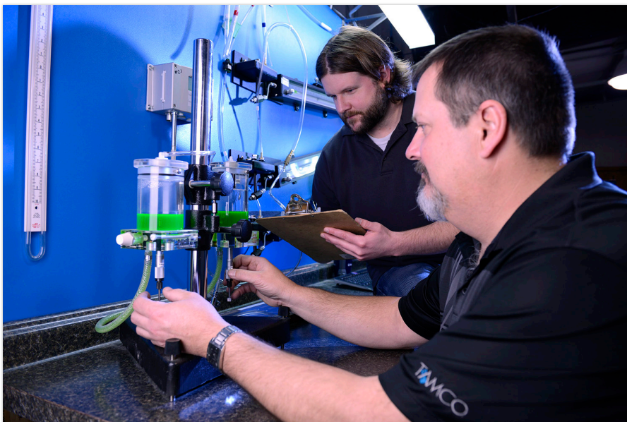
Verifying manometer calibration, function, and accuracy.
