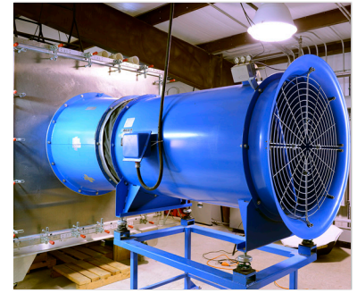
Fan connected to airtight test chamber
