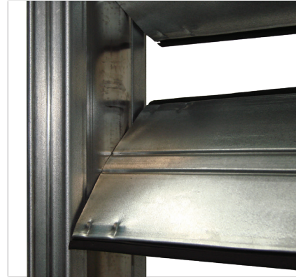
More rigid stainless steel seals require additional torque and are affected by thermal expansion as temperature increases
