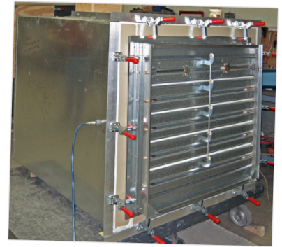
Test damper installed on thermal hot box
