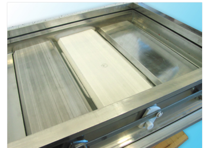
Leading competitor's thermally broken frame damper on dry ice.
