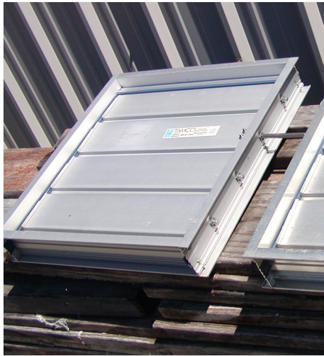
Damper has been in full sunlight for nearly eight years.
